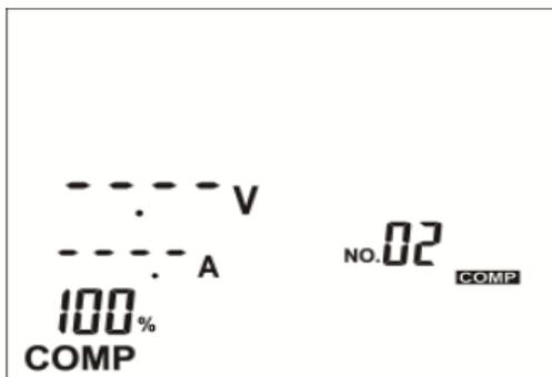
15. Press comp
