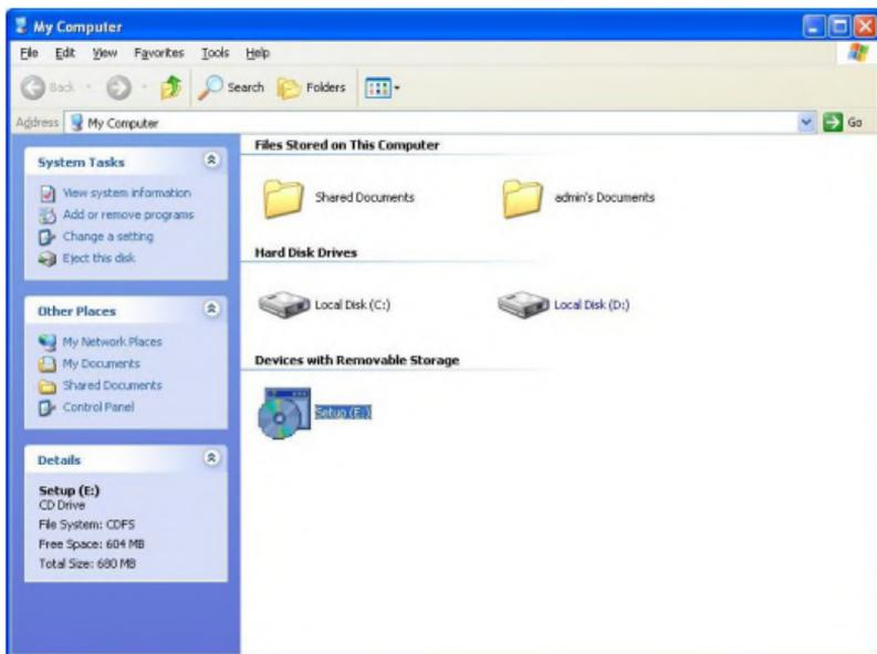
2. Select the USB drive to be installed, which is PL-2303 Drive Installer.exe, click twice on the left key of the mouse to install the USB driver.
