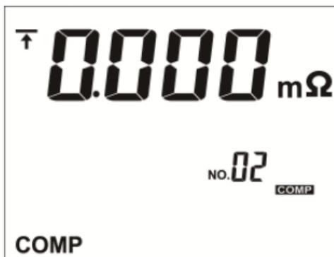
10. If select option to adjust comparator high limit resistance mode, Press comp
