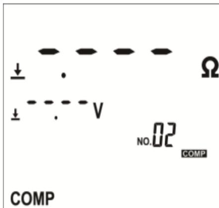
2. Press comp
