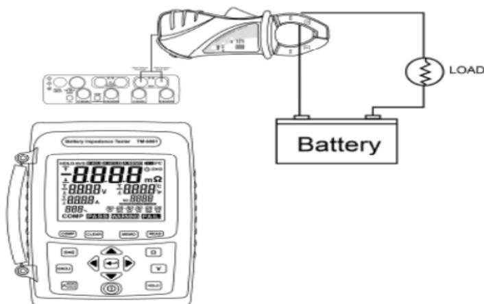
1. Connect the current probe to meter :
