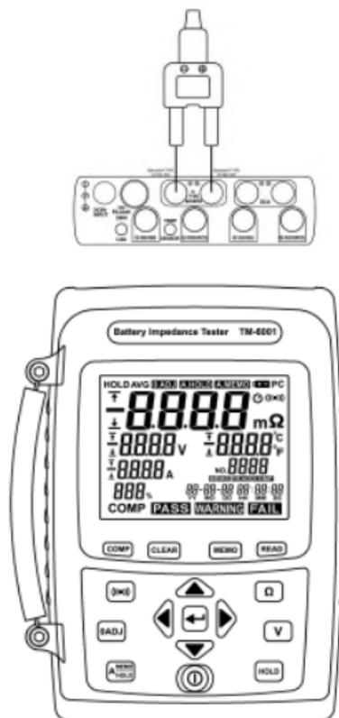
1. Insert the banana plug adapter T10 with correct + plug into K-Type sensor + JACK, and – plug into K-Type sensor – JACK
