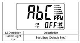
Before starting the carbon dioxide self-calibration function, please first place the device in a well-ventilated environment and provide sufficient power. The self-calibration function takes 180 hours (approximately 7.5 days); during this period the power of the device cannot be turned off. Suggested optimal carbon dioxide concentration is between 400-500 PPM.
