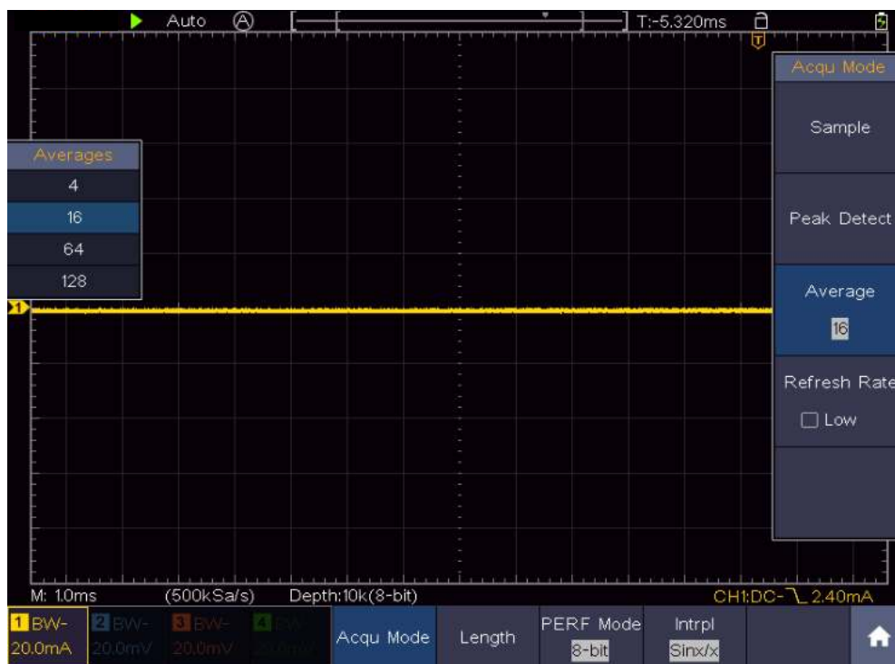
Figure 7-5 Reduce Noise level by using Average function
