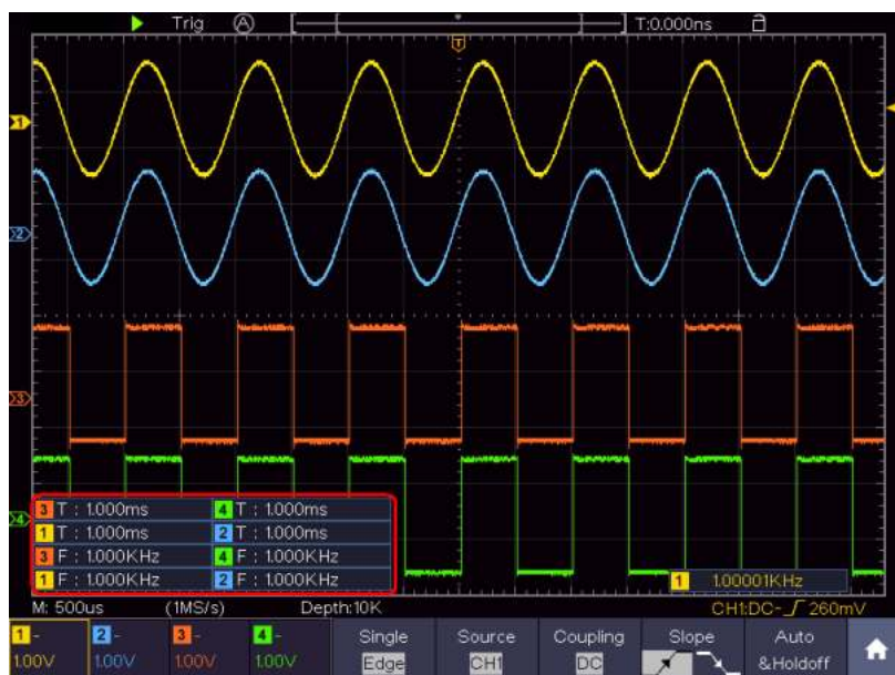
Figure 7-1 Measure period and frequency value for a given signal
