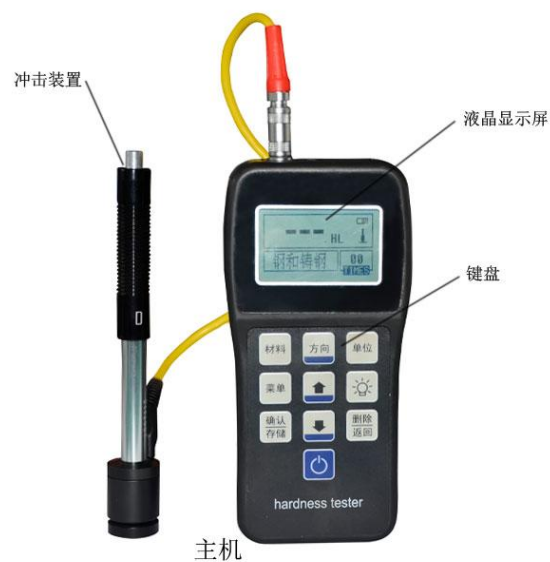
1. Host 2. Impact device 3. Keys 4. LCD screens
