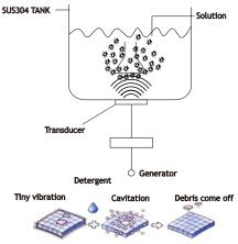
crevices, cleaning them thoroughly and consistently. Ultrasonic cleaning is extremely effective in removing dirt and grime which would normally require tedious manual cleaning. It is used to clean a wide variety of instruments and mechanical parts , returning them to almost "brand new" condition without damage to delicate parts.
