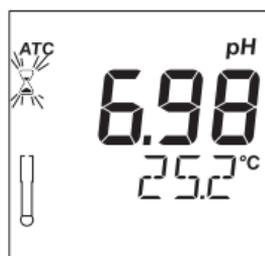
The LCD displays the pH value (automatically compensated for temperature) on the primary LCD, while the secondary LCD displays the sample temperature.
