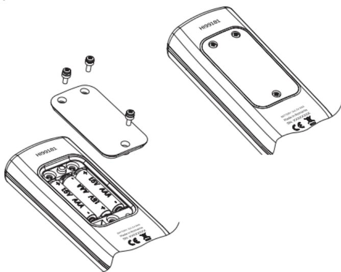
Replace the three 1.5V AAA alkaline batteries located in the battery compartment, observing the indicated polarity.
