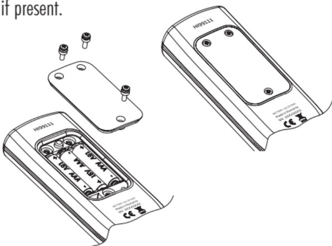
Replace the three 1.5V AAA alkaline batteries located in the battery compartment, observing the indicated polarity.
