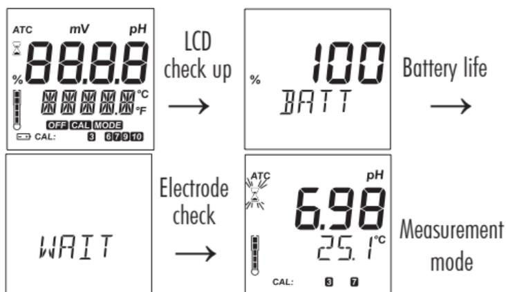
*Note: The meter detects the presence and the type of the probe at its input.*
