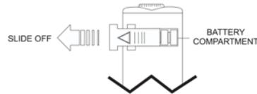
Batteries should only be replaced in a non-hazardous area and using the battery type specified in this instruction manual.
