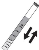
In order to avoid reagent leaking and to obtain more accurate measurements, close the cuvette first with the supplied HDPE plastic stopper
