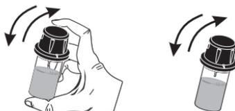
In order to avoid reagent leaking and to obtain more accurate measurements, close the cuvette first with the supplied HDPE plastic stopper
