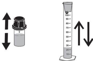
In order to avoid reagent leaking and to obtain more accurate measurements, close the cuvette first with the supplied HDPE plastic stopper
