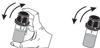
(c) The mixing method is indicated with “shake vigorously” using one of the following icons:
