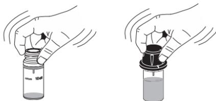
In order to avoid reagent leaking and to obtain more accurate measurements, close the cuvette first with the supplied HDPE plastic stopper
