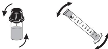
In order to avoid reagent leaking and to obtain more accurate measurements, close the cuvette first with the supplied HDPE plastic stopper
