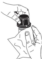
Shaking the cuvette can generate bubbles in the sample, causing higher readings. To obtain accurate measurements, remove such bubbles by swirling or by gently tapping the cuvette. Do not let the reacted sample stand too long after reagent has been added. For best accuracy, respect the timings described in each method.
