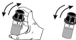
In order to avoid reagent leaking and to obtain more accurate measurements, close the cuvette first with the supplied HDPE plastic stopper
