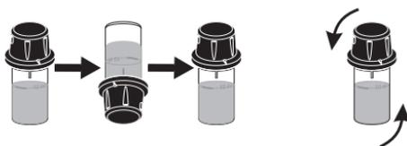
In order to avoid reagent leaking and to obtain more accurate measurements, close the cuvette first with the supplied HDPE plastic stopper
