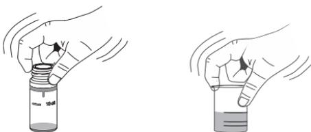
In order to avoid reagent leaking and to obtain more accurate measurements, close the cuvette first with the supplied HDPE plastic stopper
