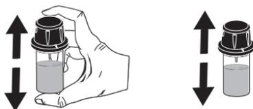
In order to avoid reagent leaking and to obtain more accurate measurements, close the cuvette first with the supplied HDPE plastic stopper
