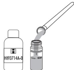
**Note:** Pay attention to the way the spoon is filled: do not press the powder; do not overfill it.
