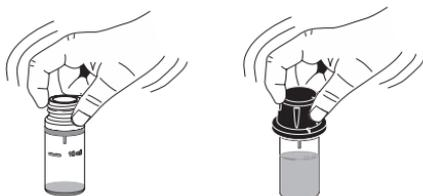
In order to avoid reagent leaking and to obtain more accurate measurements, close the cuvette first with the supplied HDPE plastic stopper
