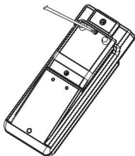
Remove the battery cover and insert the new batteries in the compartment while paying attention to the polarity.
