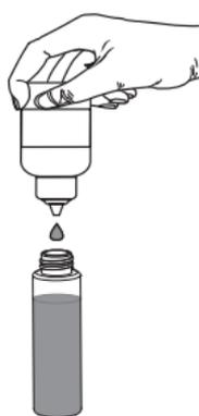
**Note:** In order to minimize any error introduced by the cuvette, it is recommended to use, during calibration, the same cuvette you are going to use to perform the measurement.
