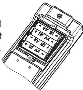
After the batteries have been installed, close the battery cover and tighten the 2 screws.
