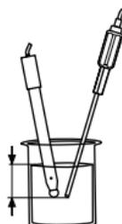
probe approximately 3 cm (1¼") into the sample to be tested and stir gently. Allow time for the electrode to stabilize.
