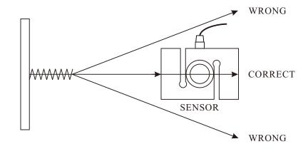
Fig 4 The Correct Measurement Direction
