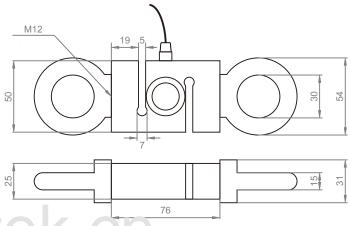
Fig 5 Shap : A d Installation Dimensions
