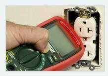
Built-in Non-Contact Voltage Detector automatically detects a live wire when the red LED is lit with audible beeper
