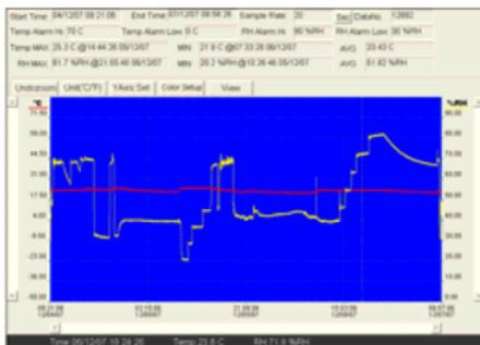
The top field show detail information of the readings (Time, Sampling rate, data numbers, Alarm Hi, Alarm Low, Max data, Min data and Avg data),
