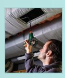
Extech Borescope features a 2.4" color monitor with video output for viewing on any monitor and a waterproof 9mm camera with bright LED lights.
