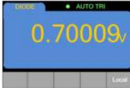
**Figure 2.6.1 Diode measurement interface**
