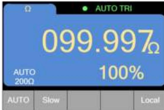
Figure 2.3.1 2-wire resistance measurement interface
