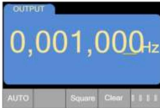
**Figure 2.8.2 Entering the frequency adjustment interface**
