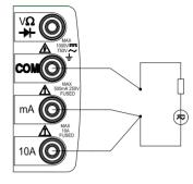
Turn off the current power, and cut off the multi-meter from the measured current.
