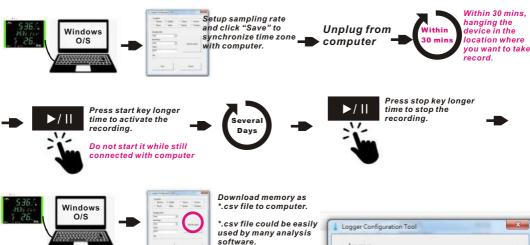
Double click "Logger configuration tool" to setup the logger. The logger configuration screen offers 8 languages to help you setup easily. The programmable parameters are sampling rate, start delay time and Logger ID.
