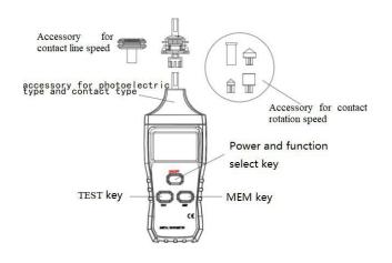
Attention: Photoelectric type measurement is recommended during measurement of high rotation speed for sake of safety.
