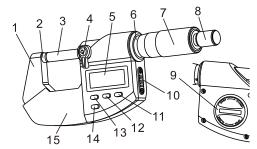
3.Spindle 1.Frame 2.Anvil 4. Locking device 5. LCD screen 6. Sleeve 7. Thimble 8. Ratchet stop 9.Battery cover 10. Data output port cover 11.HOLD/DATA button (Measured values hold on screen/data collect) 12.mm/in button 13.ORIGIN button (0 position setting) 14.ON/0/ABS button 15.Insulant pad
