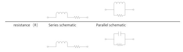
Note: generally, the series equivalent model is used for low impedance parts and the parallel equivalent model is used for high impedance parts.
